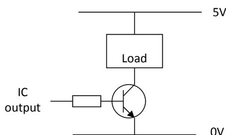
Fig B – Transistor turned off
